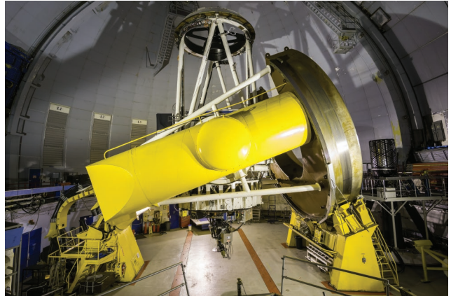
The Canada-France-Hawaii Telescope, with a 3.6-metre primary mirror. The yellow structure is the mount, which allows the telescope to point in any direction across the sky.
